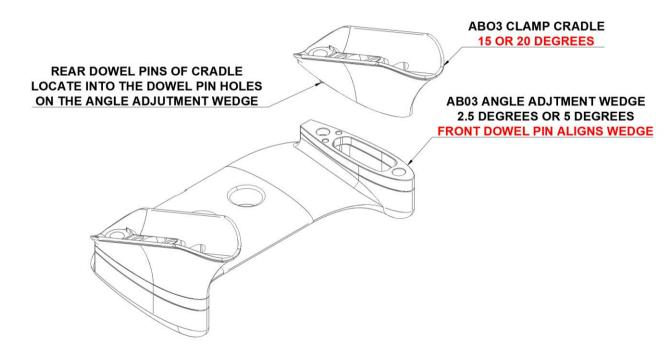
NOTE: Install with the dowel pins facing down.
