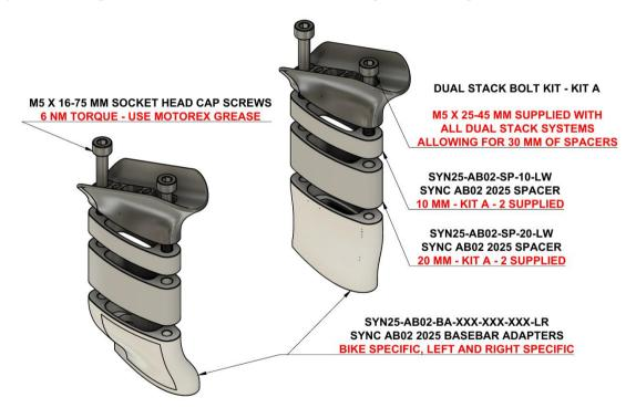
Note: Spacer Kit B (+30 mm) is available during checkout and includes Bolt Kit B (for up to 60 mm spacer height).
